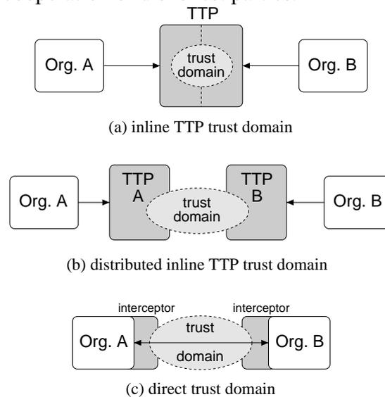
**Figure 3. Trust domains using trusted interceptors**
