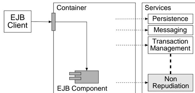
**Figure 6. J2EE-based component architecture with non-repudiation**
