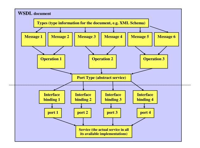
Figure 1.3: The structure of a WSDL document example
