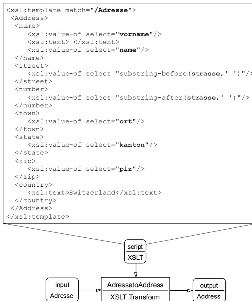
Figure 9: An alternative, equivalent representation based on XSL of the visual mapping in Figure 8 (top). The style sheet can also be invoked from an ADAPT process (bottom).
