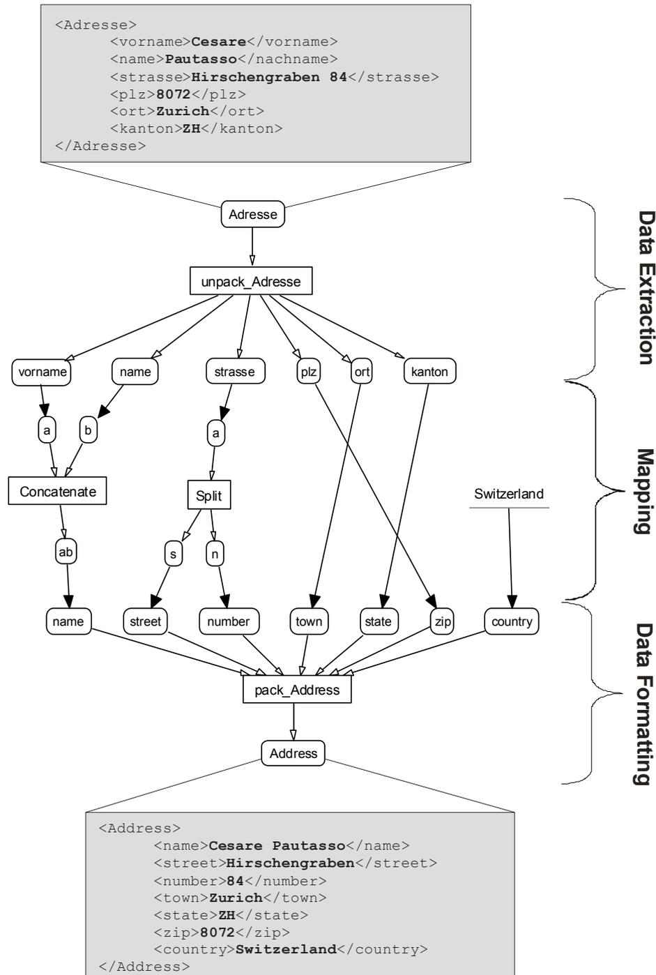
Figure 8: Example of a visual mapping between two XML complex types representing postal addresses: from a Swiss (top) to an American syntax (bottom).
