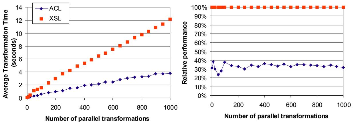
Figure 10: Absolute (left) and relative (right) performance of the ADAPT Composition Language (ACL) compared with an equivalent XSL transformation, for a variable number of transformations running in parallel.
