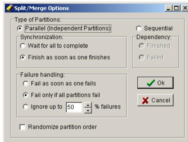
Figure 3: A screenshot of ADAPT showing the options which control the behavior of the Split/Merge operators. With them the developer can finely control if alternative services should be invoked in parallel, or sequentially. And, in the first case, if failures in invoking some of them should be ignored.
