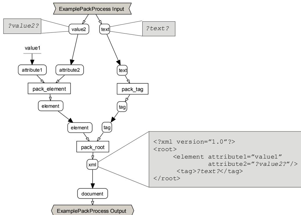
Figure 5: Example of using the XML manipulation operators to build an XML document.
