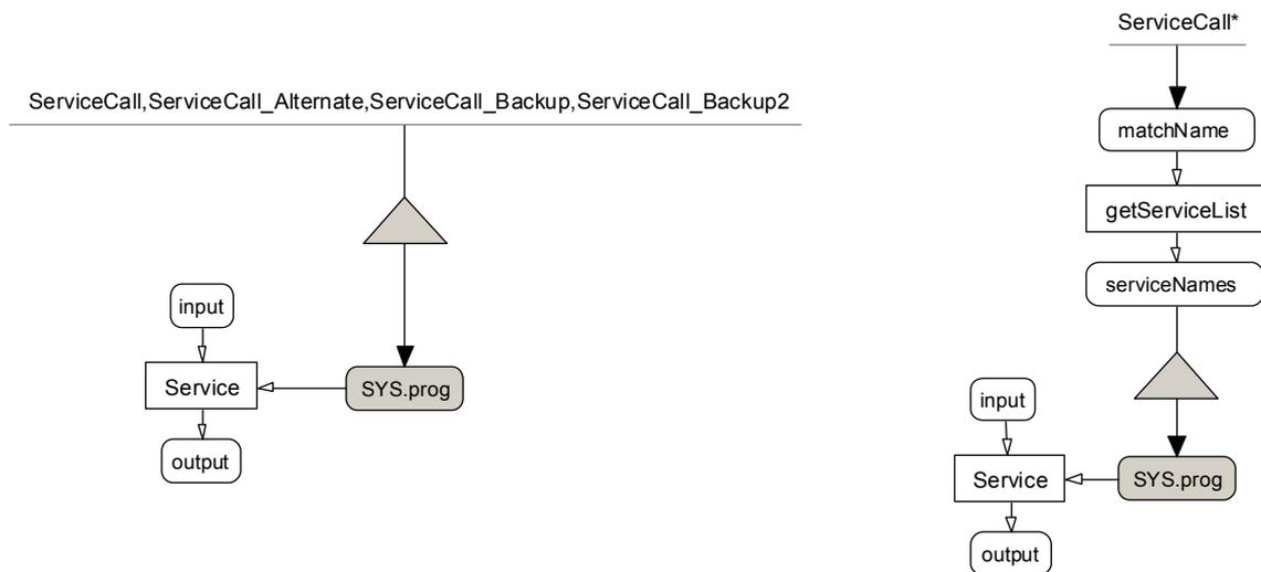
Figure 2: This data flow diagram represents the parallel invocation of the same four services of Figure 1. In the static implementation (left) the list of services is hard coded, while in the dynamic implementation (right) the list of services is retrieved at runtime. The split operator (triangle) can be configured so that the invocation will complete as soon as one of the services will respond successfully (Figure 3).
