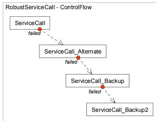
Figure 1: This chain of four Service invocations is traversed as each call fails. ADAPT attempts to contact the four alternative, equivalent services in the order specified by the control flow graph drawn by the developer.
