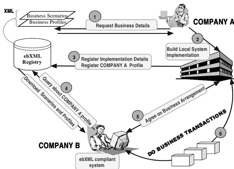
Figure 1.5: ebXML architecture
