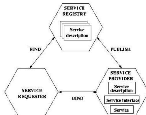
Figure 1.1: The IBM WS architecture
