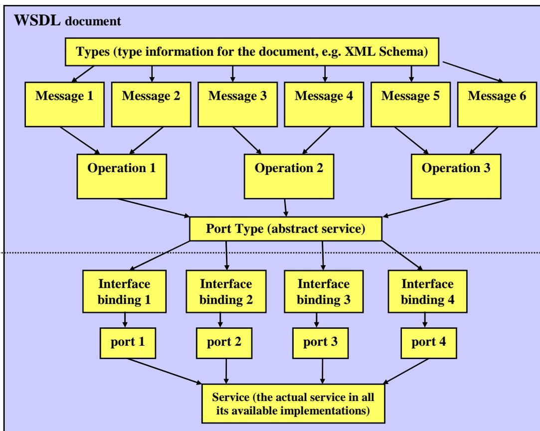
Figure 1.3: The structure of a WSDL document example
